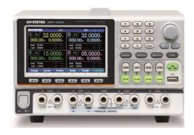
high program resolution (1mV/0.1mA) and read back resolution (0.1mV/0.1mA), but also features optimal low-ripple noise characteristics  $\leq$  350uVrms/ $\leq$  2mArms and output transient recovery capability  $\leq$  50uS. Independent output on-off switch is provided for each channel.
